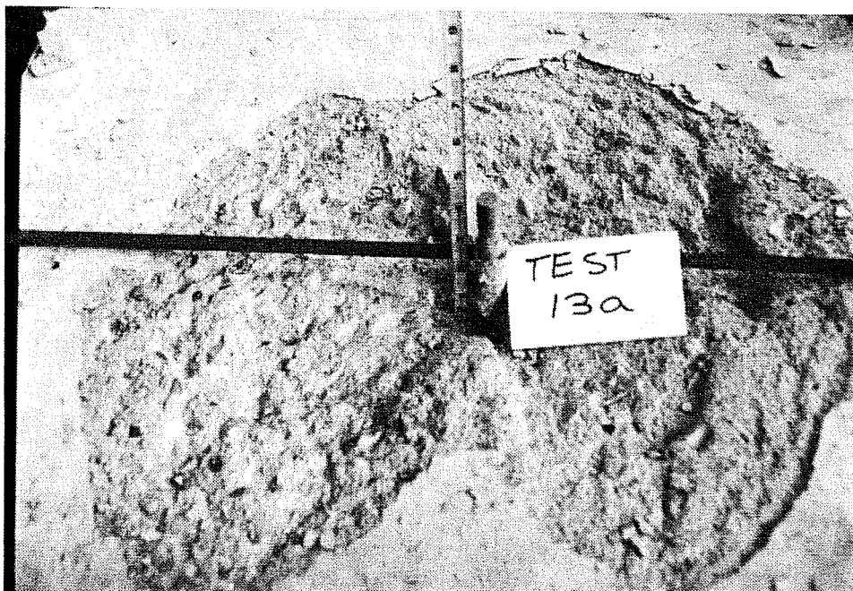
Fig. 6.6 Mode 4 Behavior (Failure of the Bond Between the Adhesive and the Concrete) for Adhesive Anchors
